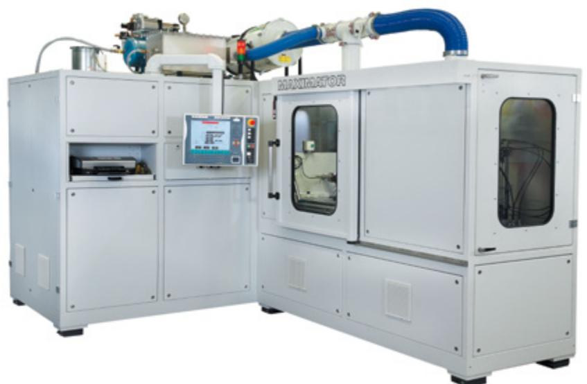
Autofrettage machine for prototypes
