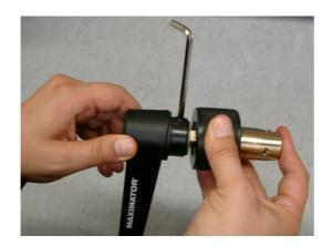
Use the supplied hexagonal offset screwdriver to loosen the headless set screw that keeps the crank handle in its position.
