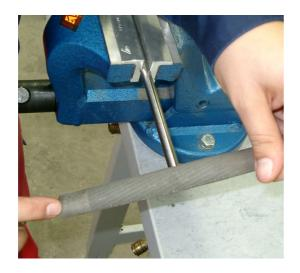
Cut the pipe to the desired length and deburr on the outside so that it can be inserted into the collet chuck of the tapering tool.
