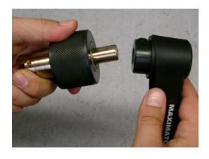
Stick the components onto the blanking die holder in the following sequence: Needle bearing → Knurled nut → Needle bearing → Crank handle.
