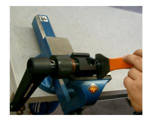
Tighten the tensioning nut with the chuck key. Make sure that all 4 springs of the chuck keys are gripping the tensioning nut slots.
