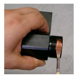
Lubricate the threads of knurled nut and base structures (We recommend use of solid lubricant. such as copper paste).
