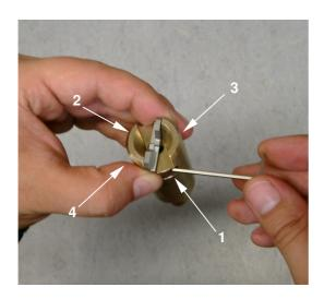
Use the hexagonal offset screwdriver to slightly tighten the headless set screws to align the blanking dies. Make sure to first tighten the headless set screws located opposite the cutting edges (see sequence in the illustration). Thus, the blanking dies with cutting edges fit closely to the blanking die holder. Otherwise the processed taper surface may be uneven.
