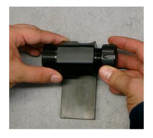
Slightly grease tensioning nut and collet chuck and screw them onto the base structure.
