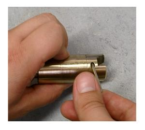
Loosen the 4 headless set screws in the blanking die holder to disassemble the blanking dies. Then remove the blanking from the blanking die holder.
