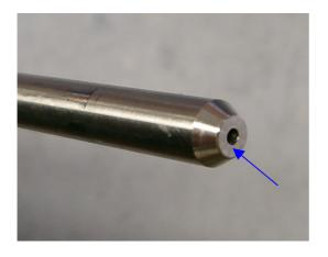
The finished pipe can be recognised by the completely machined face side of the pipe. The taper surface must be free from any damage, such as indentations or scratches. If this is not the case, the pipe can be simply re-machined.
