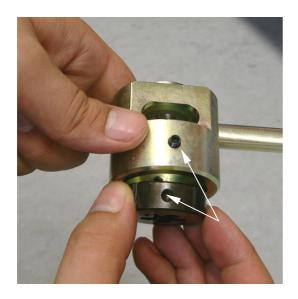
Insert the die stock and guide bush into the tool body and secure with headless set screws. Align the components in such a manner that the headless set screws grip into the recesses.
