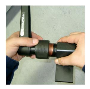
Insert the blanking die holder into the base structure and screw the knurled nut on with a few rotations. Now the coning tool is ready for use.
