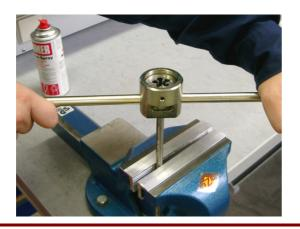
Slightly press down the tool and start the threading operation (in counterclockwise direction). Rotate the tool briefly in clockwise direction during the threading process in order to break the chip and apply more cutting oil.
