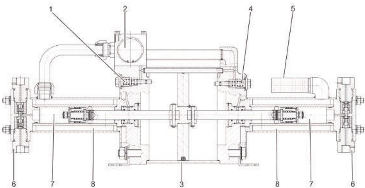
Fig. Maximator booster, type DLE 15
